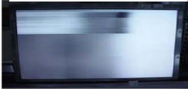
Horizontal Block Gate TAB IC Defect
