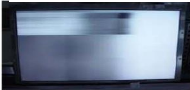
Horizontal Block Gate TAB IC Defect
