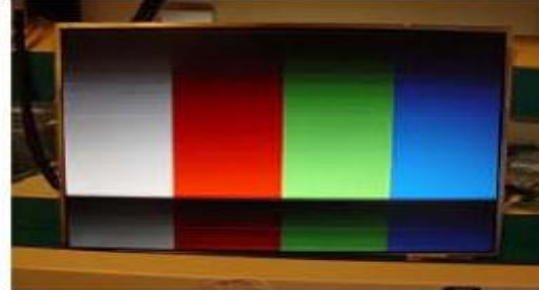
Horizontal Block Gate TAB IC Defect
