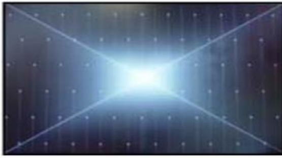
Solder defect, Short/Crack
