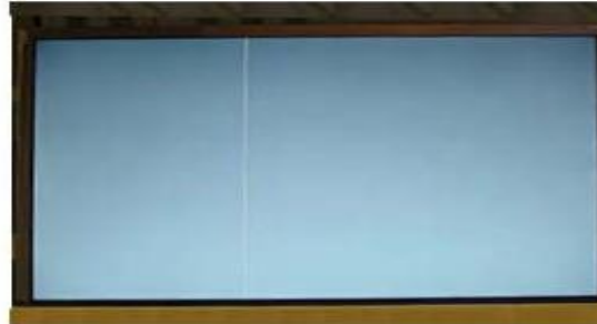
Vertical Line Source TAB IC Defect
