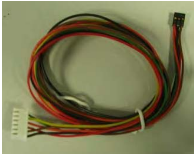
Fig2: Cable from programming module board to chassis
