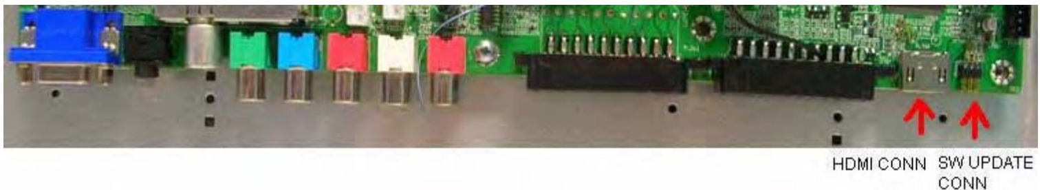
Fig1: Position of the software update connector at the backside of TV
