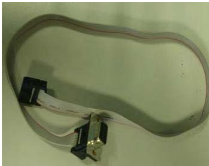
Fig5: Cable from module board to PC COM port
