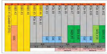
Figure 3-1. HSIO Muxing on SKL PCH U
