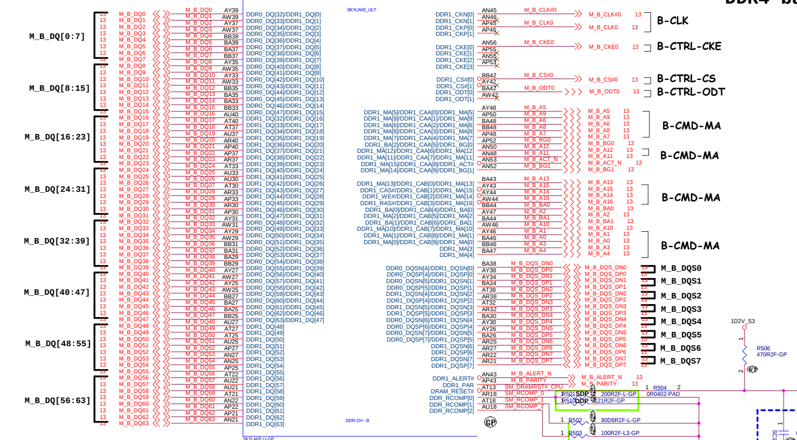
Figure 5-14. SKL U DDR4 6L Mixed SO-DIMM and Memory Down x16, T-Daisy Topology Memory Down Strobe/Data/Reset/RCOMP Signal Topologies
